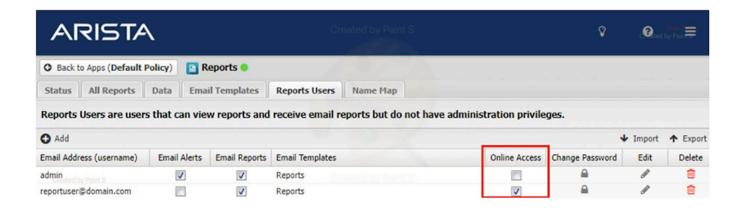
The above picture shows the configuration panel for user access. The "report" user has "Online Access" checked, which is required in order to be vulnerable.
