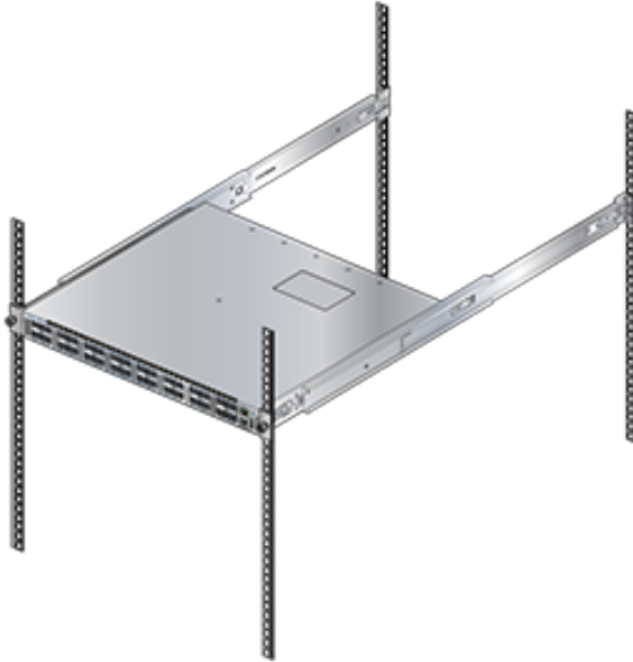
Figure 13: Attaching the Switch to the Rack Posts
