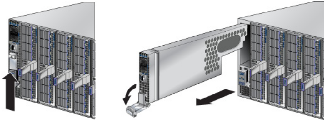
Figure F-4: Supervisor Module Maintenance
