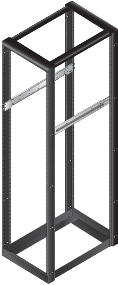
Figure 2: Rack Rails Installed
