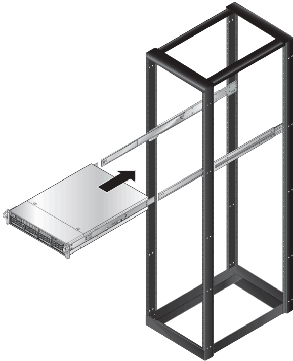
Figure 3: Installing the Appliance into a Rack
