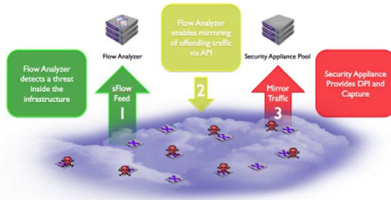
Figure 4: Automating detection and focused capture using open APIs
