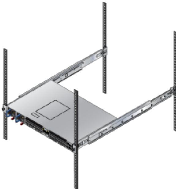
Figure 9: Attaching the Switch to the Rack Posts
