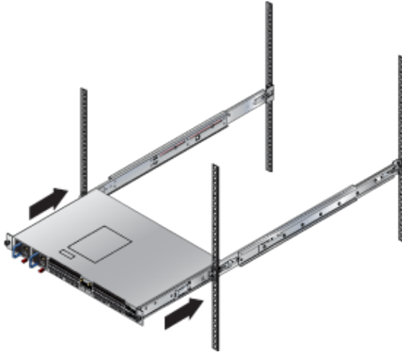
Figure 8: Inserting the Switch onto the Rails
