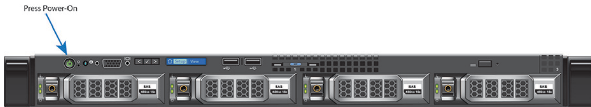
Figure 6: Power On Button Location
