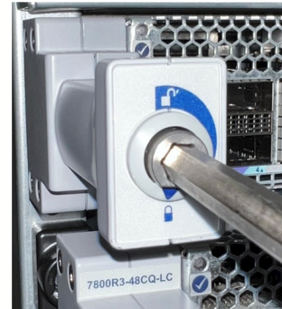
Ejector locked when fully injected
