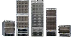
The R4-Al generation of Arista's flagship 7800 series of modular systems implement an Al optimized packet pipeline in addition to the field-proven fully-scheduled, 100% fair internal architecture, and delivers support for up to 460 Tbps of 800G Al focused connectivity. Offering up to 576 ports of 800G, or 1152 ports of 400G, the 7800R4-Al is the most efficient and performant single-box solution for clusters up to 144 nodes and the ideal spine system for large 2- or 3- tier topologies.
