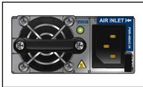
Figure 4-1: Power Supply Socket
