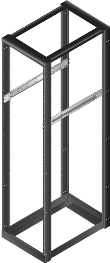
Figure 3-2: Rack Rails Installed
