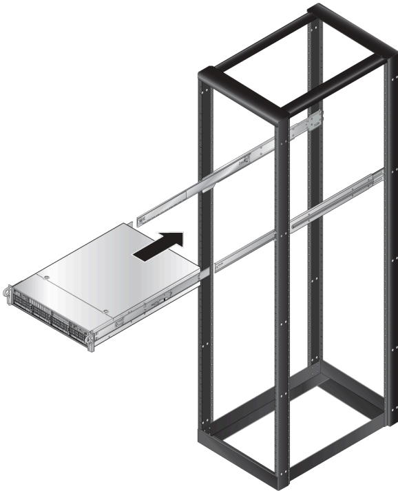
Figure 3-3: Installing the Appliance into a Rack
