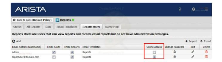
The above picture shows the configuration panel for user access. The "report" user has "Online Access" checked, which is required in order to be vulnerable.
